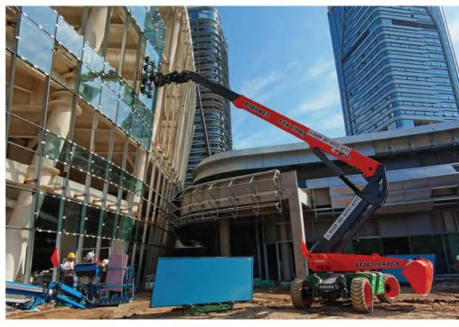
The earlier model of Dingli electric glass attachment boom lift, the BT2612ERTGS, offers a maximum suction capacity of 1,200 kg. This machine can handle 13 large, heavy glass panels per day on average.
