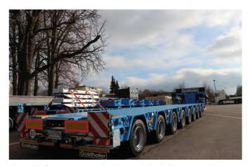
The Goldhofer MPA 8 semitrailer has an axle load of 15.6 t per axle line. So, each vehicle can easily handle operations with a total weight of more than 150 t. The semitrailer also features a very low loading height.
