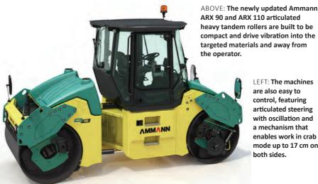
heavy tandem rollers are built to be compact and drive vibration into the targeted materials and away from
