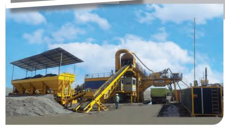
innovative modular construction (the entire plant is built inside ISO shipping containers for safe, economical transportation) allowed for fast installation and commissioning after arriving on the jobsite.
