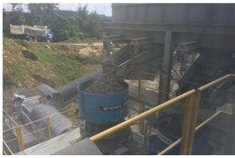
ALL IMAGES: The Terex MPS plant helps build the Pan Borneo Highway in Malaysia, by producing aggregates to be used for road base throughout the project.
