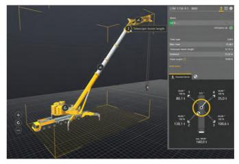
The displayed data are determined by the same calculation logic system as the live data generated by real mobile and crawler cranes.
