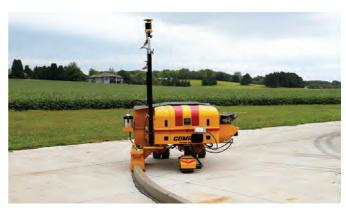
Gomaco has introduced the world's first battery-powered slipform curb machine. the CC-1200e.
