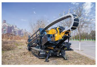
TOP AND ABOVE: The Vermeer D60S HDD has 266.9 kN of thrust and pullback and 12,202.4 Nm of rotational torque.
