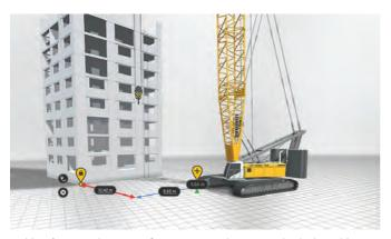
Liebherr's Crane Planner 2.0 features a new distance tool, which enables objects to be positioned relative to each other with centimetre precision.
